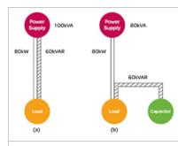
Figure 3. In this example, supplying the reactive power locally with a capacitor brings the power factor to unity and reduces the power supplier's apparent load from 100 kVA to 80 kVA.
